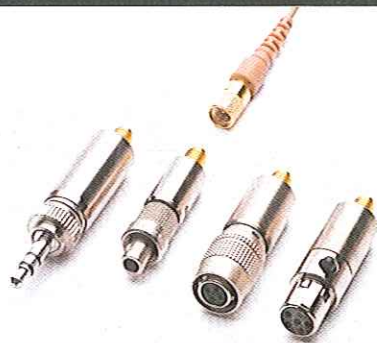
The detachable connectors interface to a wide variety of wireless transmitter packs or an XLR input.
